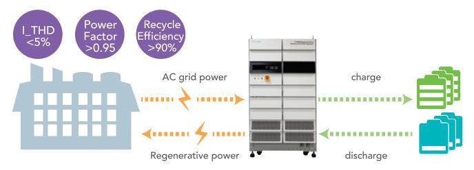
■ Smooth AC current waveform and real-time phase transition when energy is regenerated to the grid. This prevents other equipment from being affected by false test results or a contaminated grid
